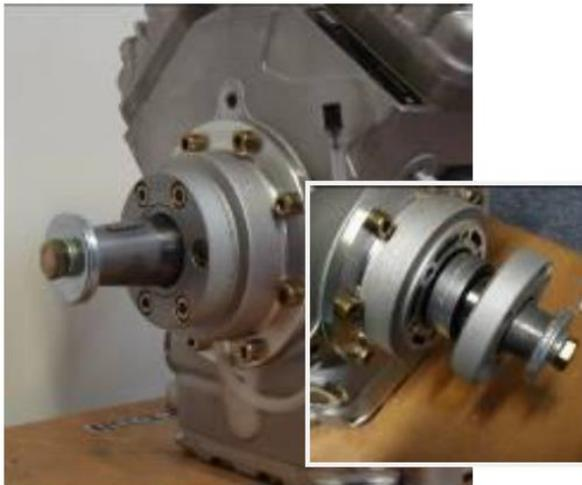
General wear of the shaft seal over time, increased oil loss from the slip ring
