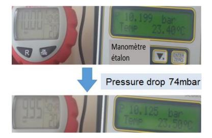
FIGURE 8. RESULT WITH A DIGITAL PRESSURE GAUGE
